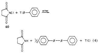
either thallium salt to give thallous chloride by an ionic mechanism should be precluded, since such a reaction would necessitate the formation of a succinimidyl cation or thallium anion. Homolytic cleavage to give phenylthio or phenylseleno radicals, succinimidyl radicals, and thallous chloride should occur.
